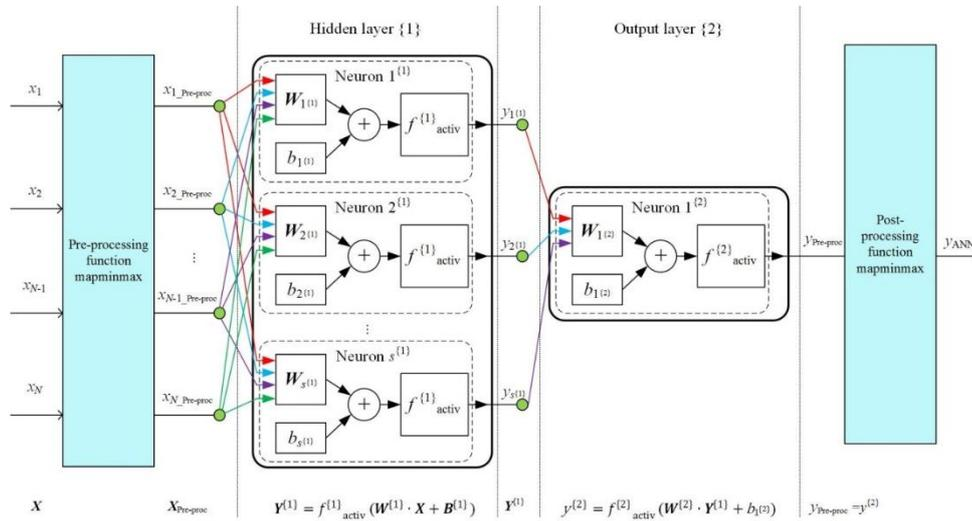
**Figure 3.** The structure of a one approach of neural network used in the study [1]
