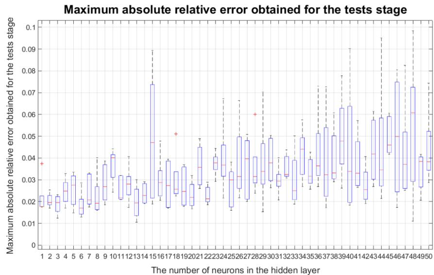
**Figure 5.** Maximum absolute relative error obtained for the neural network structure with a certain number of neurons in a hidden layer
