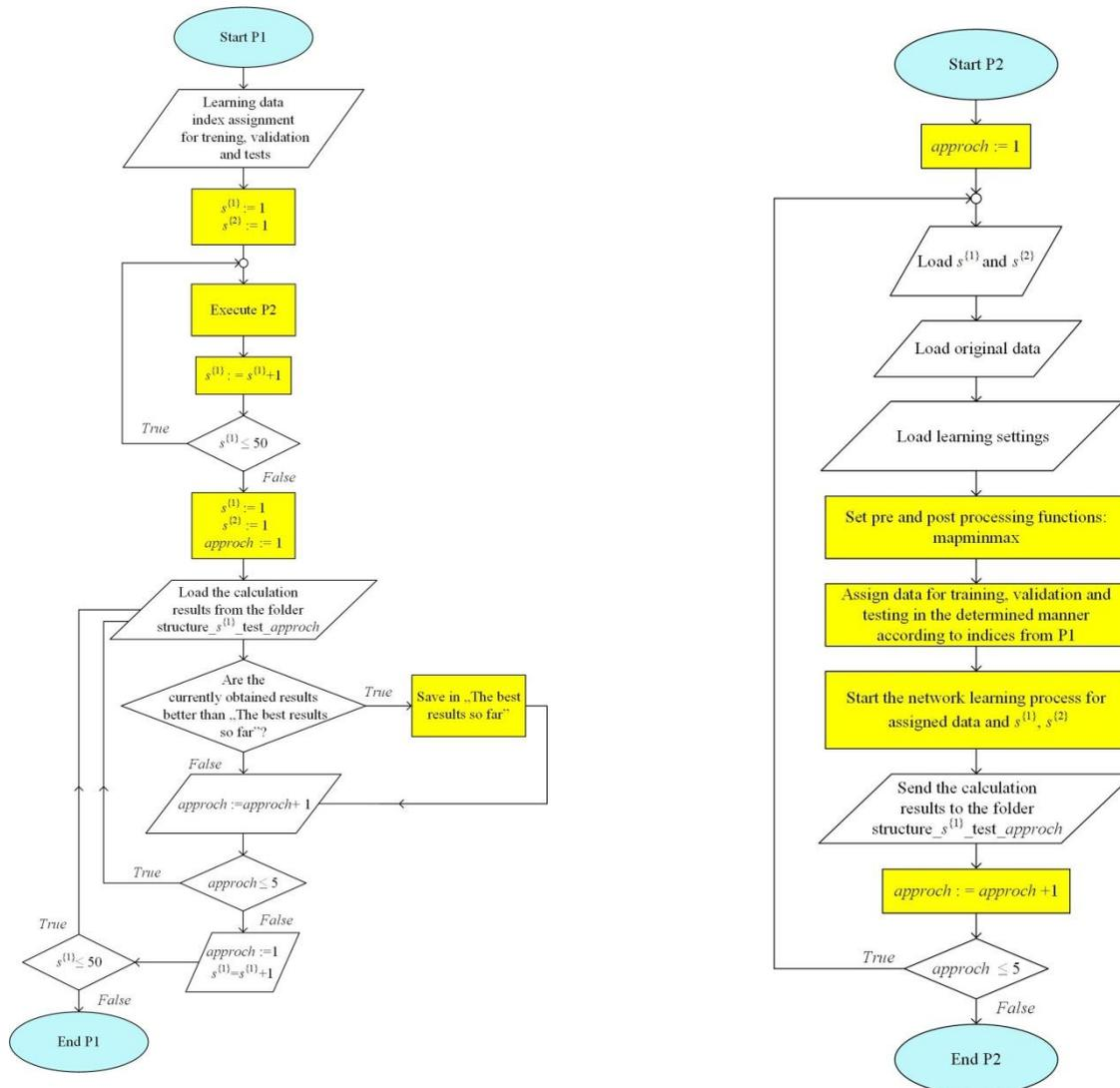
**Figure 2.** The algorithm for identification of the best possible dimension of the matrix of the model describing the examined physical phenomenon: (a) Parent procedure P1; (b) Nested procedure P2 [1]
