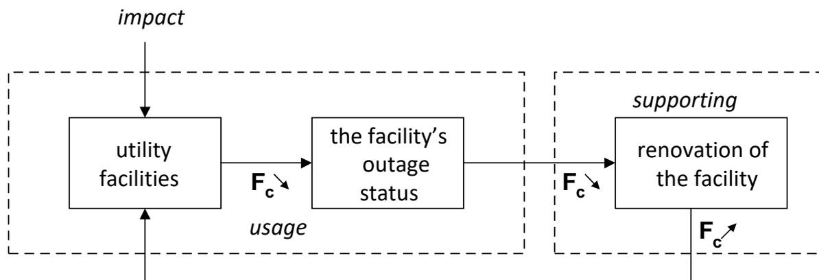
Figure 1: Diagram of the technical facility operation process.
