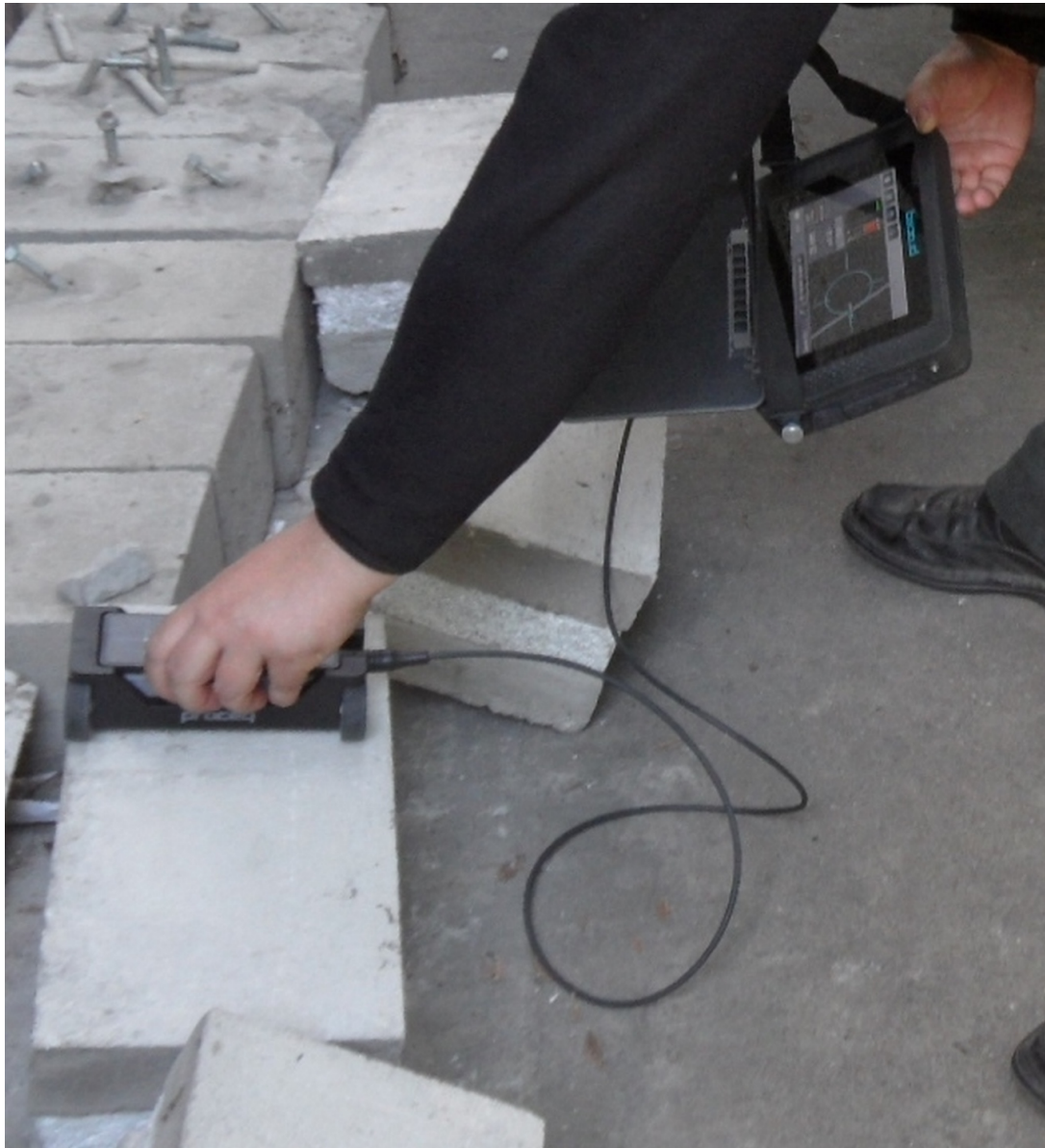
Figure 3. Preparation of the Profometer PM-650 for testing.
